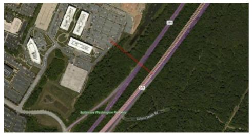
Figure 6: Example of a ventilation/exit shaft (red line to private property from main alignment)
